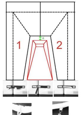
place the pole vault front panels (01 and 02 see the drawing on page 4) around the pole vault box, so as the distance between the rear edge of the box and the landing area pads (a) is 15 cm, make sure that all the Velcro<sup>®</sup> pads adjoin properly. Next main segments 03 and 04 should be linked together
