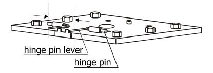
After that the post is ready to be installed on the base trolley. Unscrew screws M20x40 (4 pcs) and remove washers 20 (4 pcs). Press hinge pin levers according to the arrows.
