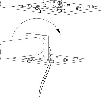
Pull out the cog belt ends from post profile and thread them through the hole in base trolley
