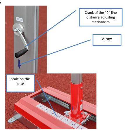
Turn the crank clockwise or counter clockwise until the blue arrow points a desired distance from "0" line on the scale installed on the stand base.
