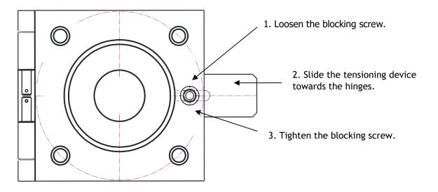
Now tighten the nuts (you have screwed temporarily in base side plates) with wrench. Correctly tensed cog belt should deflect no more than 2 cm approx. when pressed with index finger. Cog belt tensioning should be done scrupulously. If cog belt is too loose, it may slip on toothed wheels in post sliding mechanism. On the other hand, when cog belt is too tense, it may cause too high resistance and load of sliding mechanism.
