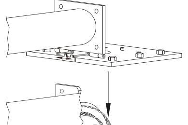
Release hinge pin levers, which spring back automatically to their working positions and connect post foot with base trolley. That pivotal joint is used to put posts in the upright position.
