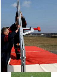
If the stand bases are not covered by the landing area and they are positioned next to it, the folded post must be rested on the 5. special support (included in the set, item 4), without the support the post will fall down and the folding mechanism will be damaged.
