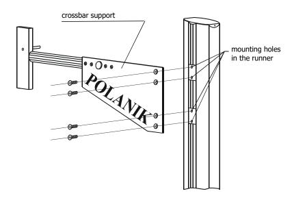
Next screw down crossbar supports to the posts while they are resting on the ground. Use 4 countersunk screws for each support. The screws are temporally mounted in the runners of the posts.
