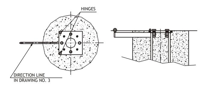
The extreme anchors (item 2, drawing no. 3 and 5, image 1) have got special reinforced arms for installing the bottom net tension cable (item 6). All supplied anchors are ready for embedding (screws are fully screwed down and their threads coated with rubber sleeves).
