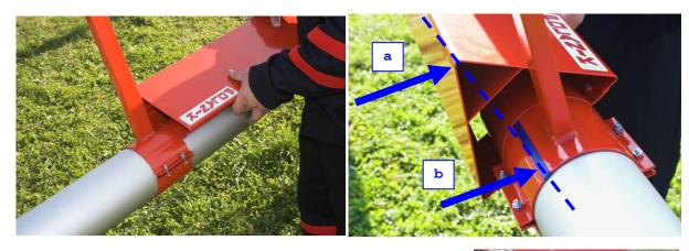
After the shield frame being fixed properly, screw the clamping rings (2) using screws (3) and washers (4).
