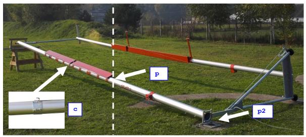
After erecting the gate and fixing its wings by following the instruction, the shields tip should aim to the center of the circle. Properly installed shields are shown below.
