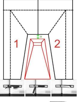
place the pole vault box surrounding pads (1 and 2 see the drawing on page 3) around the pole vault box, so as the distance between the rear edge of the box and the landing area pads (a) is 15 cm, make sure that all the Velcro<sup>®</sup> pads adjoin properly, next attach front panels 3 and 4,
