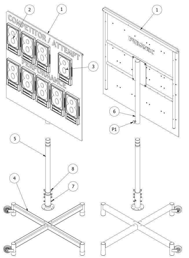
Drawing no 2. Assembly of the performance board T9-S271.
