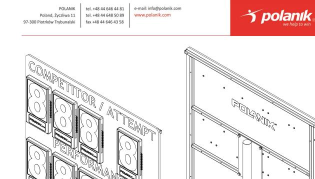
Drawing no 1. Factory installed subassembly of the performance board T9-S271.
